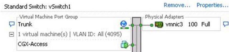
The physical network adapter would be required to connect to the trunk port on the physical networking switch.
