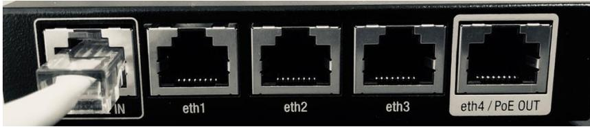
Adapter 1 is not protected, so if this subnet needs protection, a second cable should be attached to Adapter 2 (eth1). Each vLinks Remote can protect 4 subnets.
